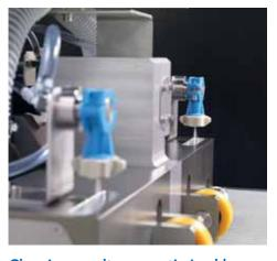
Cleaning results are optimised by the finely tuned interaction between the cleaning chemical, the water, and the brushes rotating in different directions.
