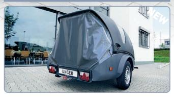
Optional protection cover for the hose reels. Robust truck tarpaulin that can be fixed on the new fixing point at the trailer frame.
